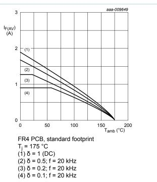
Fig. 9. Average forward current as a function of ambient temperature; typical values
