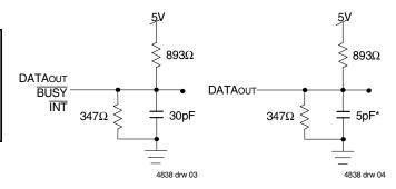
Figure 1. AC Output Test Load
