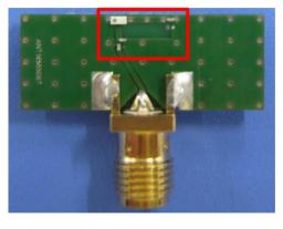
PCB size : 25mm x 10mm x 1mm Antenna area : 6 x 2.5 mm
