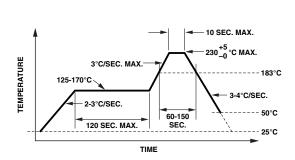
Recommended SnPb reflow soldering profile.
