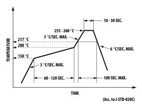
Recommended Pb-free reflow soldering profile.
