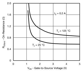
On-Resistance vs. Gate-to-Source Voltage
