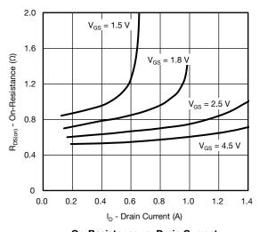
On-Resistance vs. Drain Current
