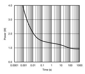
Single Pulse Power, Junction-to-Ambient <sup>a</sup>
