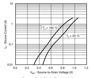
Source-Drain Diode Forward Voltage
