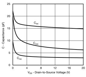
Capacitance vs. Drain-to-Source Voltage
