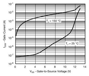
Gate Current vs. Gate-Source Voltage
