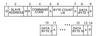
Figure 25. Block Write to a Register
