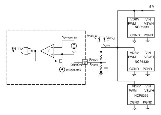
Figure 12. DRVON and DrMOS Supply UVLO Circuit
