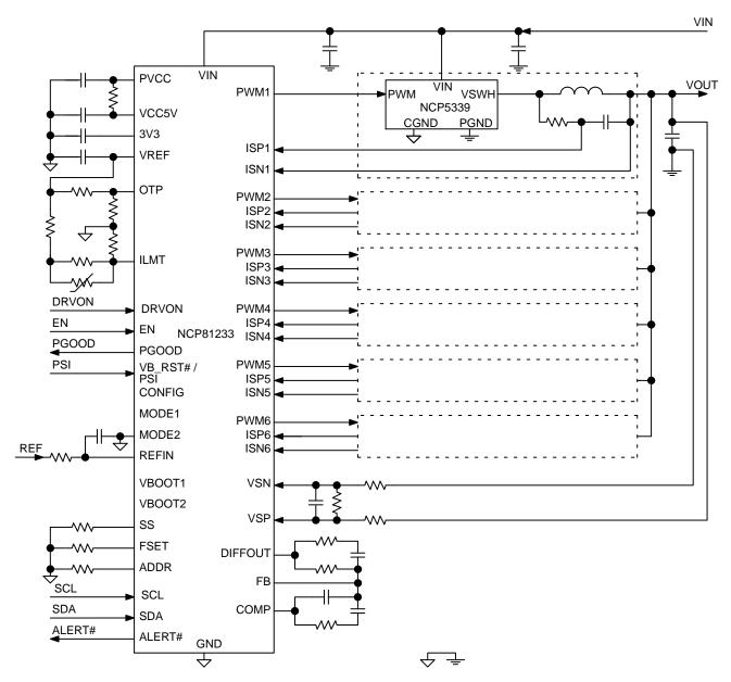
Figure 3. Typical Application Circuit with External Reference Input
