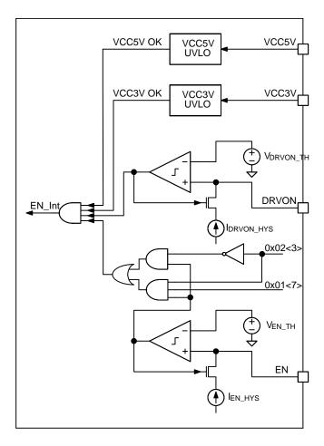
Figure 9. Enable, DRVON and UVLO
