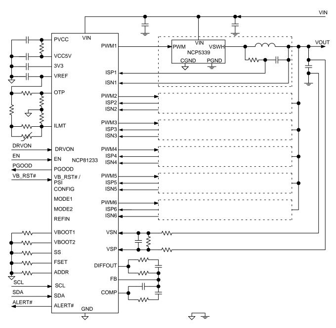
Figure 2. Typical Application Circuit with Programmed Boot Voltage
