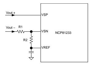
Figure 15. Adding Offset Voltage in Output
