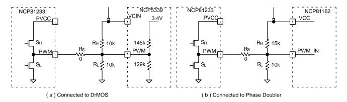
Figure 13. PWM Connections to DrMOS and Phase Doubler
