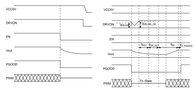
Figure 7. Timing Diagram of Power Down Sequence
