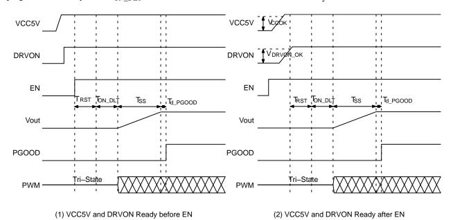
Figure 6. Timing Diagrams of Power Up Sequence
