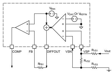
Figure 14. Output Voltage Sensing and Regulation
