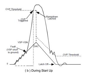
Figure 17. Function of Latch-Off Over Voltage Protection
