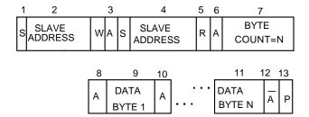
Figure 28. Block Write to a Command Coder
