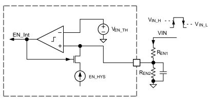
Figure 11. Enable and Input Supply UVLO Circuit
