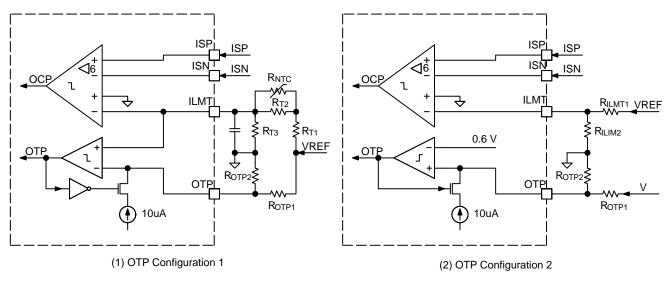
Figure 18. Over-Current Protection and Over-Temperature Protection
