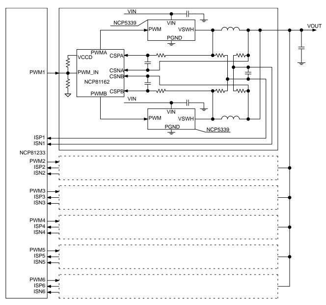
Figure 4. Application Circuit with Phase Doublers
