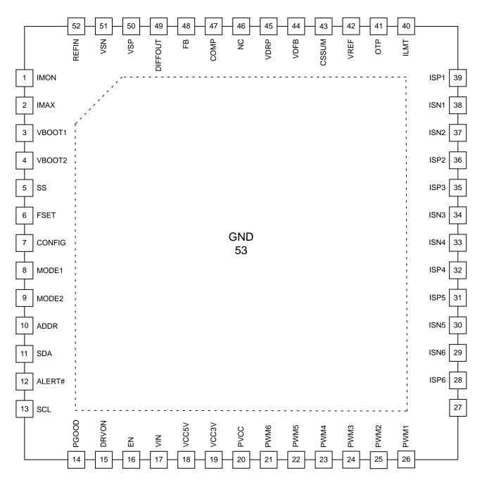
Figure 1. Pin Configuration
