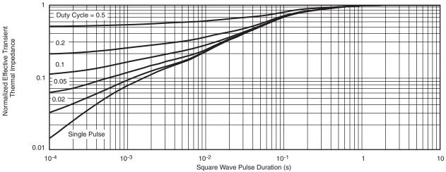
Normalized Thermal Transient Impedance, Junction-to-Foot
