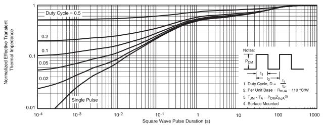
Normalized Thermal Transient Impedance, Junction-to-Ambient
