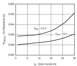
On-Resistance vs. Drain Current and Gate Voltage
