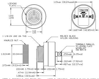
NOTE A: TERMINALS-032 BRASS TIN PLATED, TAPPED FOR #6-32 SCREW. TWD #6-32 NICKEL PLATED BRASS SCREWS INCLUBED. WILL ACCEPT 1/4\* QUICK CONNECT. NOTE B: MOUNTING- REMOVE BLACK PLASTIC NUT AND INSERT THREADED FRONT THROUGH 1.25' HOLE PUNCHED IN PANEL, IF DRIENTATION IS NEEDED, NOTE LOCKING FLATS ON DRAWING, SCREW NUT BACK ON. DO NOT OVERTIGHTEN.
