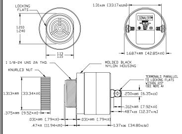
NOTE A: TERMINALS-.032 BRASS TIN PLATED, TAPPED FOR #6-32 SCREW. TWO #6-32 NICKEL PLATED BRASS SCREWS INCLUDED. WILL ACCEPT 1/4' QUICK CONNECT. NOTE B: MOUNTING- REMOVE BLACK PLASTIC NUT AND INSERT THREADED FRONT THROUGH 1.25' HOLE PUNCHED IN PANEL, IF DRIENTATION IS NEEDED, NOTE LOCKING FLATS ON DRAWING, SCREW NUT BACK ON. DO NOT OVERTIGHTEN.
