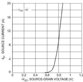
Fig. 8 Forward Drain Current vs. Source-Drain Voltage
