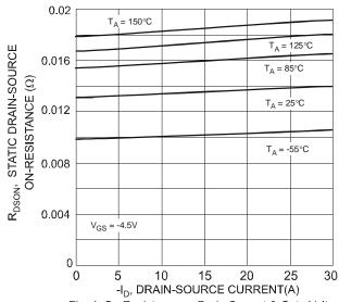
Fig. 4 On-Resistance vs.Drain Current & Gate Voltage
